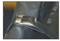
Tap down latch ears. This band is secure. Remove excess banding from Mandrel.
