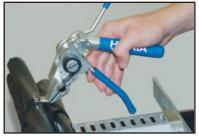
When desired level of band tightness is achieved, Tool Nose is flush with latch.
