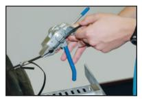
Position the BT-200 in loading position (ratchet handle forward) then place the band through Tool Nose and Winding Mandrel. Make sure there is plenty of band through the Mandrel.
