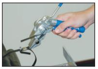
Grip Ratchet Handle and pull back toward Handle to tighten band. Repeat this action until band is at desired tightness.
