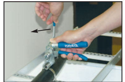
With a firm grip on the CT-7, grasp Cutter Handle with other hand.
