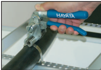
Repeat this action until band is at desired tightness.
